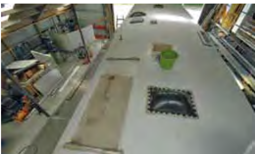
From top: Dave and Karen Gomm; Selwyn and Lynda Buckett; The two couples were ecstatic to see the results!; All hands on deck! Three motorhome roofs in one day is nothing for the Lifestyle Motorhomes team; The Buckett's RV roof scrubbed and prepared for application.
